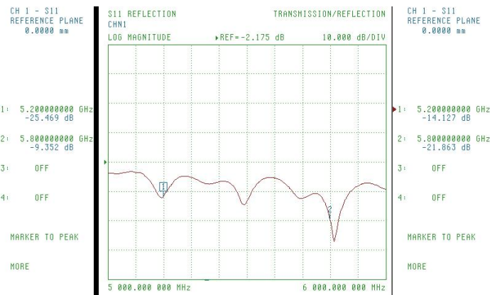
Return loss with 4.4mm separator
