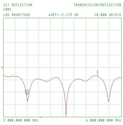
Return loss with 5.3mm separator
