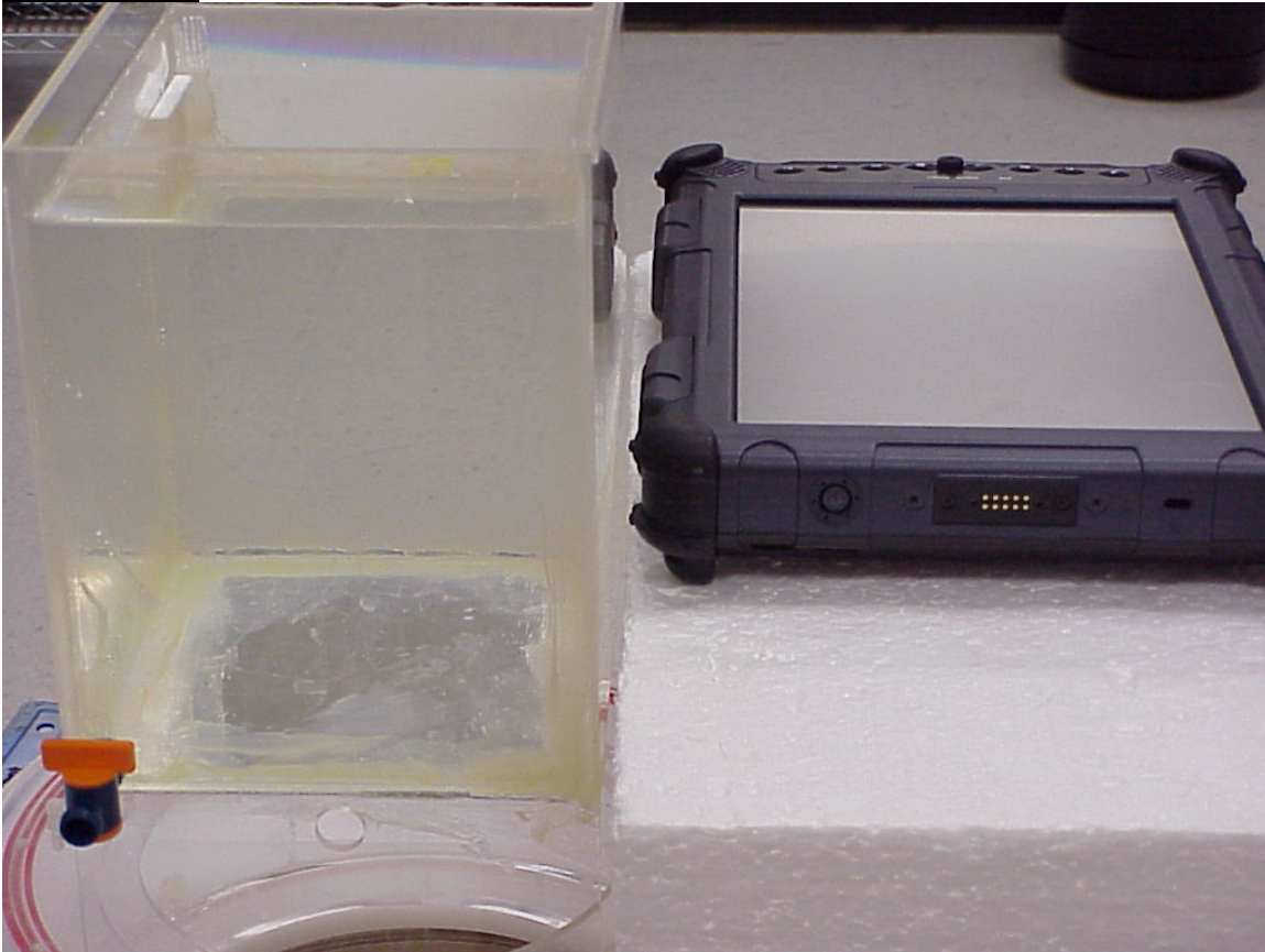
Photo 4. GPRS antenna bystander position
