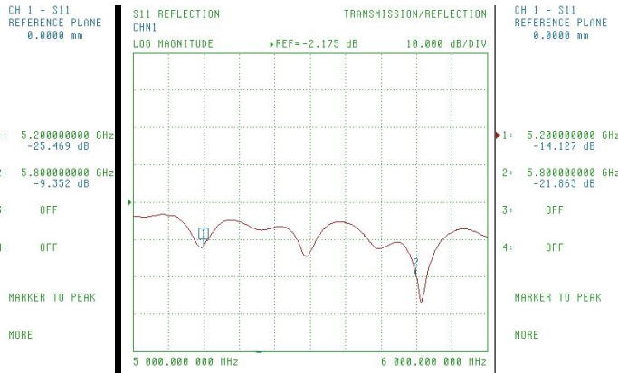
Return loss with 4.4mm separator
