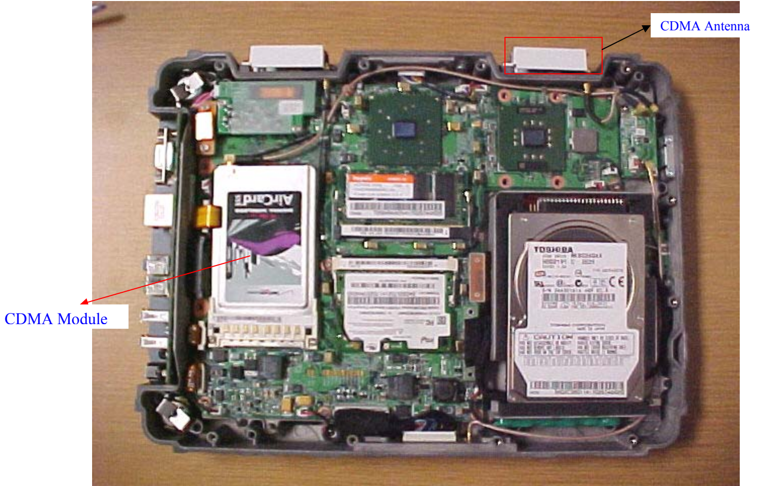
EUT – Internal view showing CDMA module
