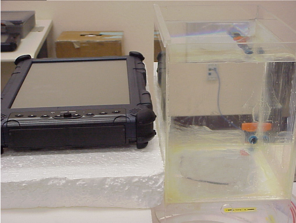
Photo 4. 2450 MHz antenna bystander position
