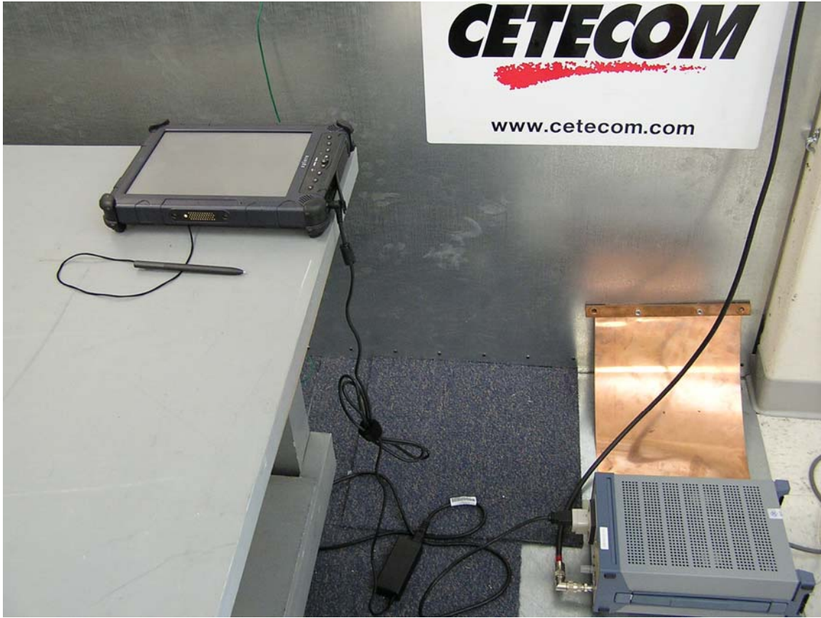
Test setup – AC Line Conducted Emissions
