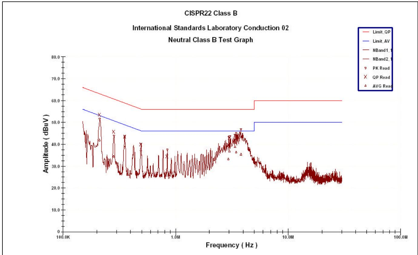
\* NOTE: During the test, the EMI receiver was set to Max. Hold then switch the EUT Channel between 1 , 6, 11 to get the maximum reading of all these channels.
