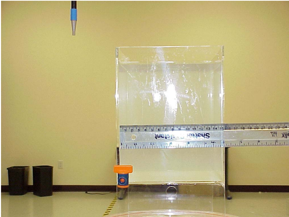
Photo 9. Photo to demonstrate 15 cm Z-axis flat phantom
