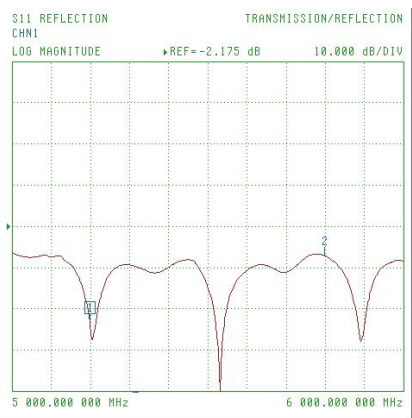
Return loss with 5.3mm separator
