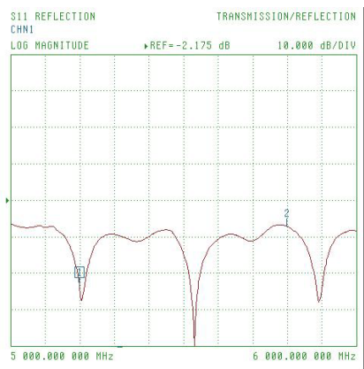
Return loss with 5.3mm separator
