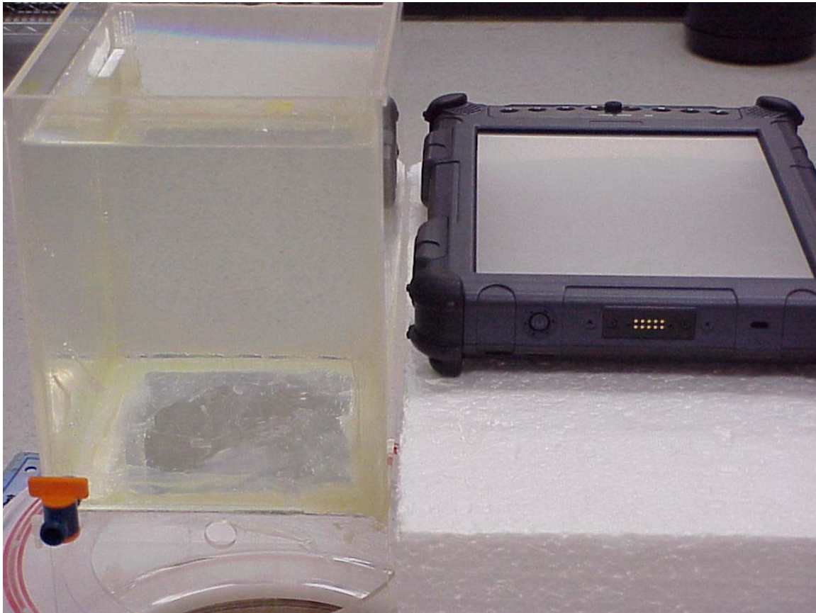
Photo 7. GPRS antenna bystander position
