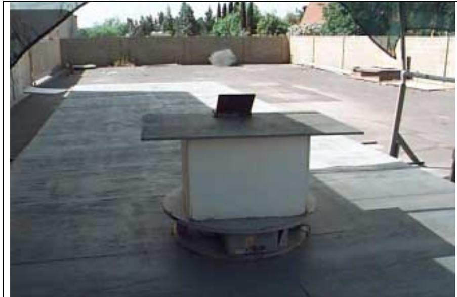
TEST SETUP: Radiated Emissions
