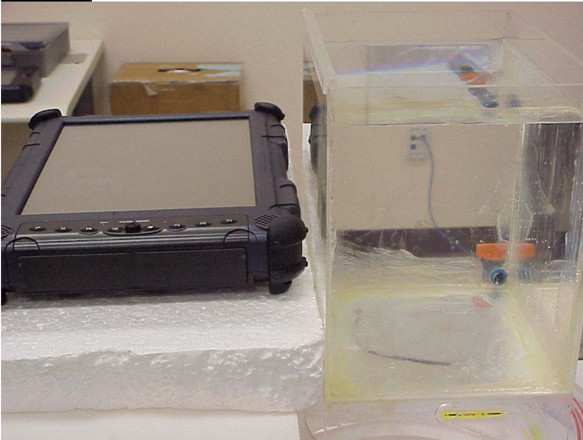
Photo 4. 2450 MHz antenna bystander position
