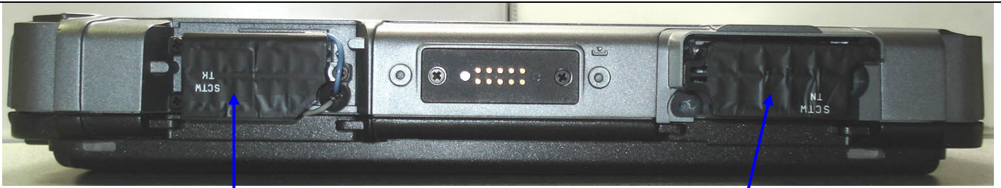
Top Edge of iX104C5 Tablet PC with WWAN "PUMP-UP" Antenna Housing removed
