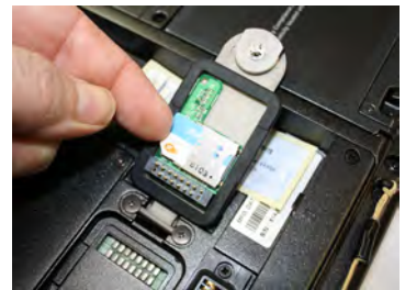
Installing a SIM card
