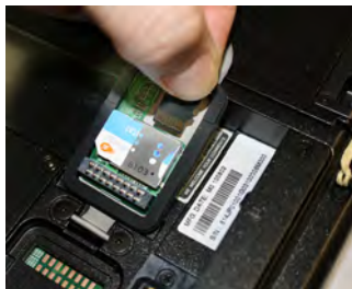
Installing a MicroSD card
