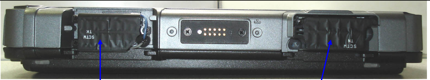
Top Edge of iX104C5 Tablet PC with WWAN "PUMP-UP" Antenna Housing removed
