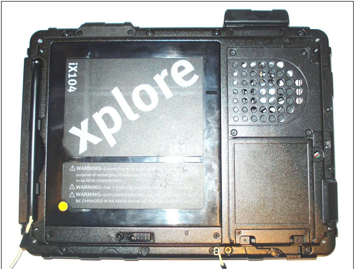
Bottom Side of Tablet PC with WWAN “PUMP-UP” Antenna Housing
