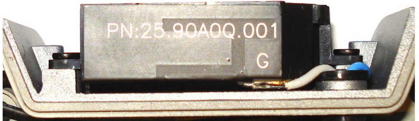
WLAN AUX (CHAIN B) TRANSMIT DIVERSITY ANTENNA HOUSING
