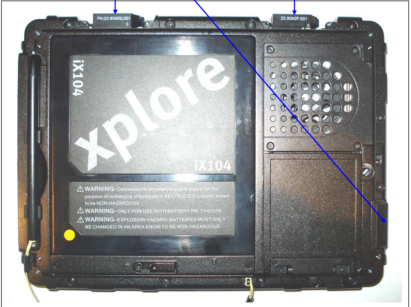
ANTENNA LOCATION(S) – BOTTOM VIEW OF XPLORE iX104C5 TABLET PC
