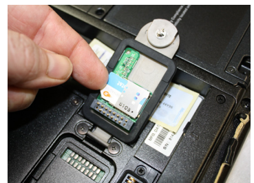
Installing a SIM card
