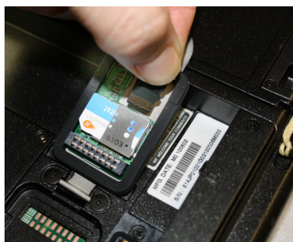
Installing a MicroSD card
