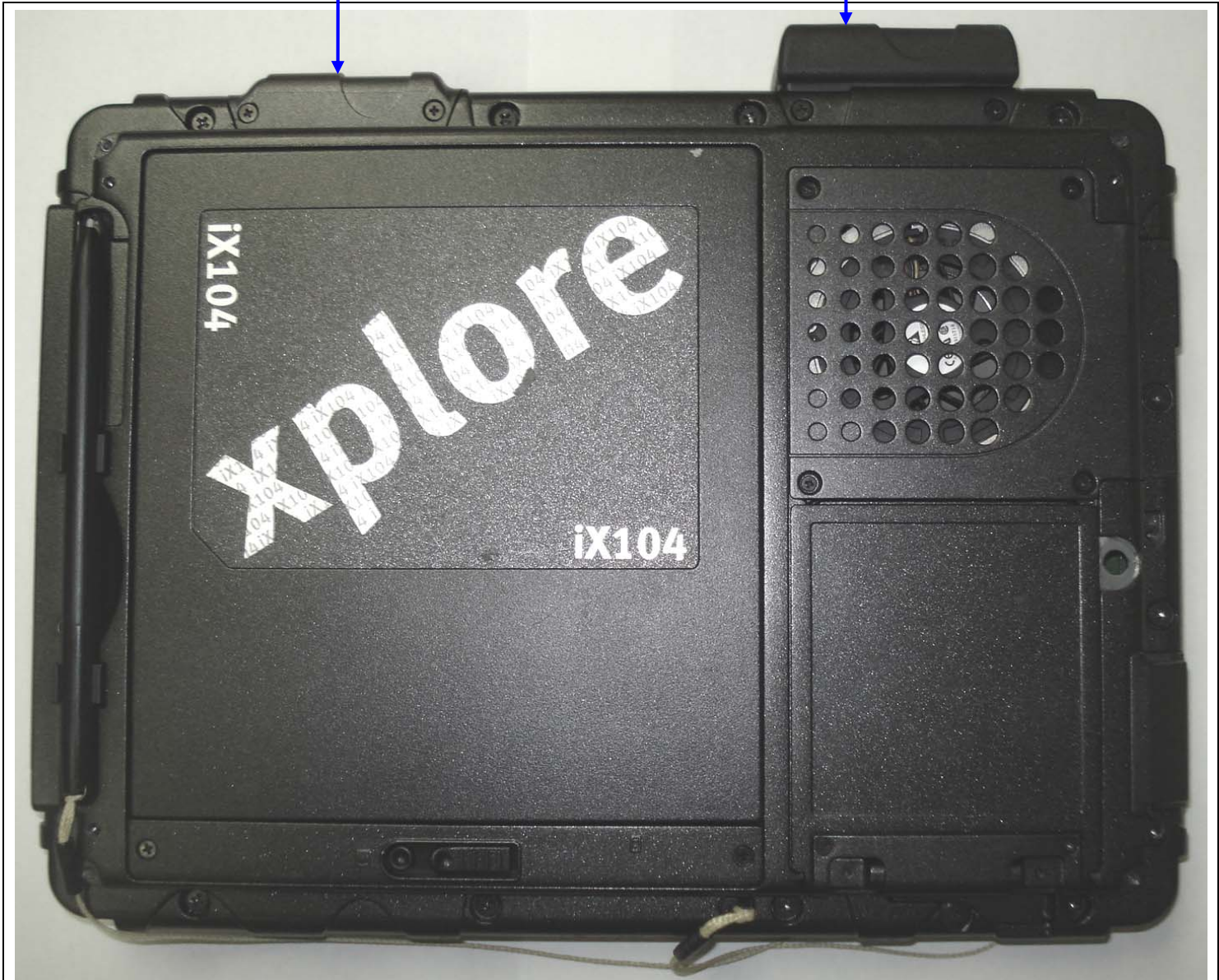
Bottom Side of iX104C5 Tablet PC with Li-ion Battery
