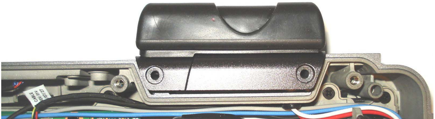
WWAN TRANSMIT ANTENNA HOUSING (“PUMP-UP”)
