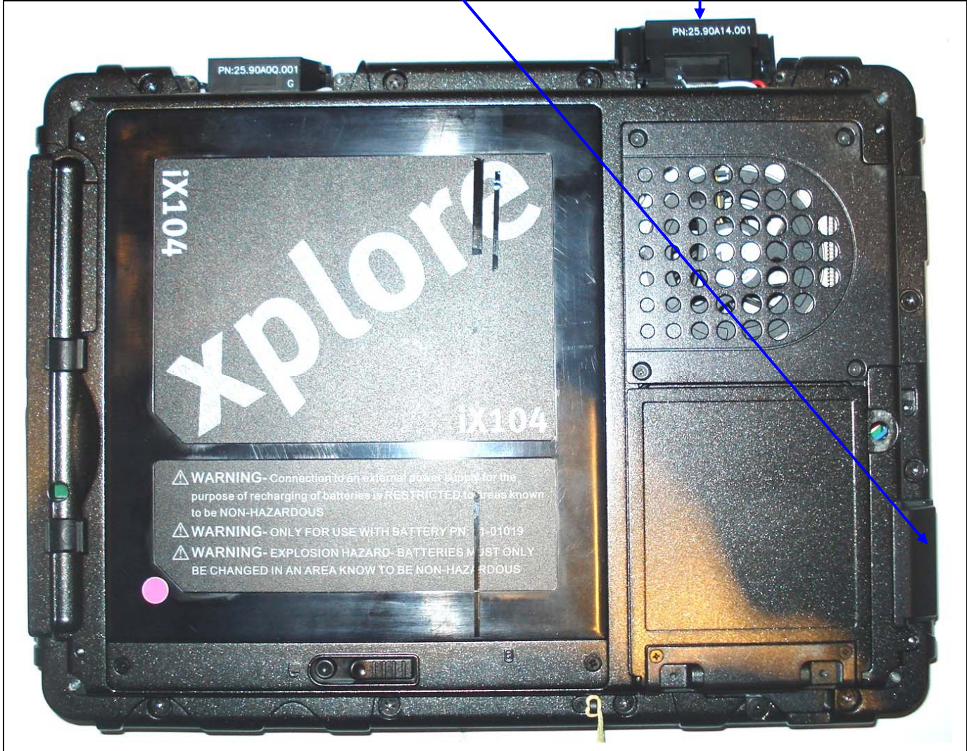
ANTENNA LOCATION(S) – BOTTOM SIDE OF iX104C5 TABLET PC
