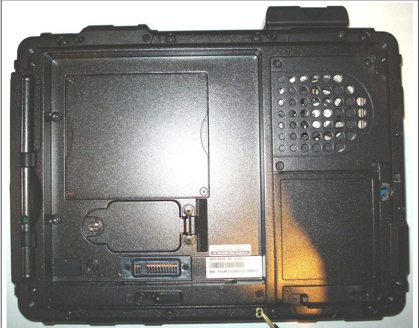
Bottom Side of Tablet PC with Li-ion Battery Removed
