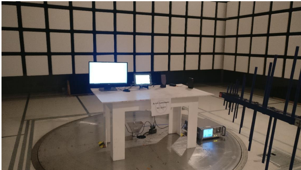
Front Radiated disturbance 30MHz - 1GHz
