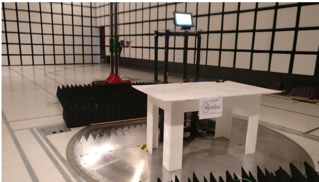
Back Radiated disturbance 1GHz - 18GHz
