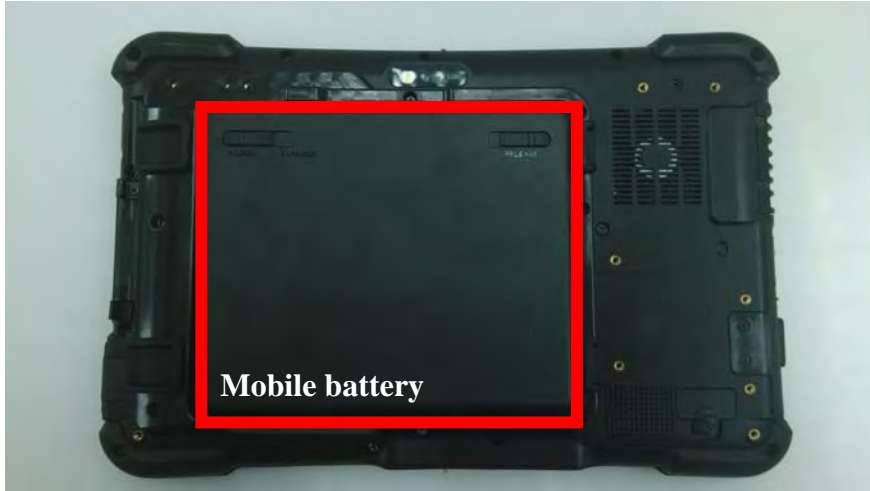
Fig.14 Back view of EUT with mobile battery (The thickness of mobile battery is 11mm)
