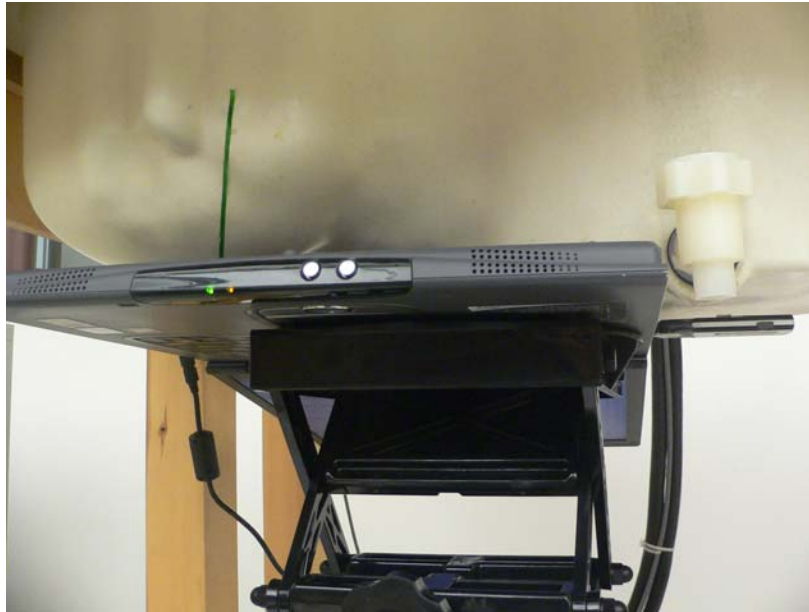
Acer laptop with DUT back touching to the flat phantom
