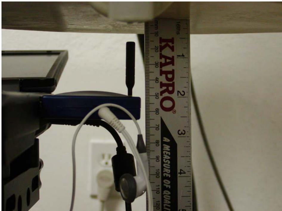
**Compal, keyboard side facing phantom, EUT top side facing phantom, antenna pointing into and perpendicular with phantom**
