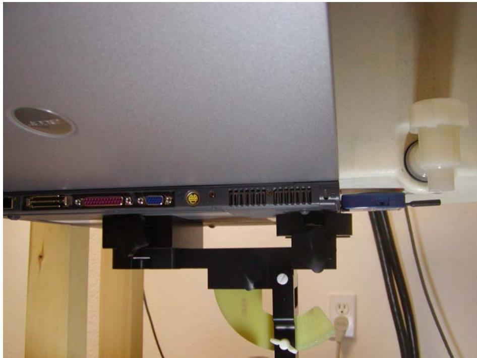
**Acer, Keyboard side facing phantom, EUT Top side facing phantom, antenna pointing into and perpendicular with phantom with headset**
