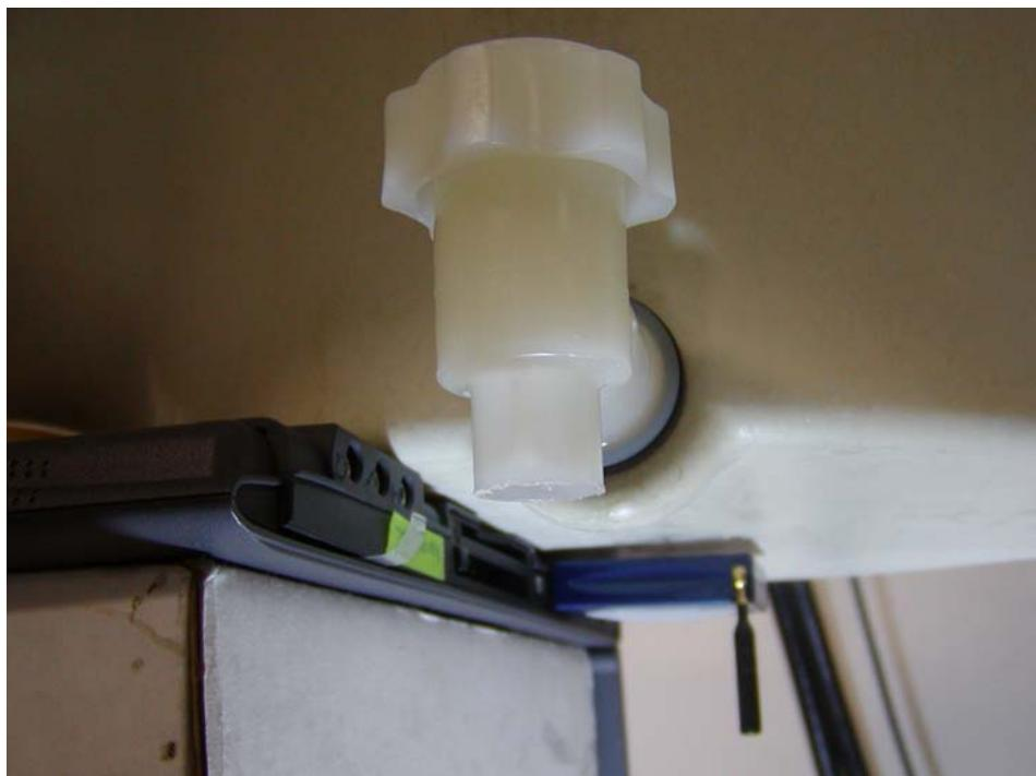
**Acer, Keyboard side facing phantom, EUT Top Side facing phantom, antenna parallel with phantom bottom with headset**
