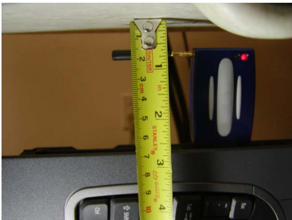
**Toshiba, Bottom side facing phantom, EUT bottom side facing phantom, antenna pointing down and perpendicular with phantom and headset**
