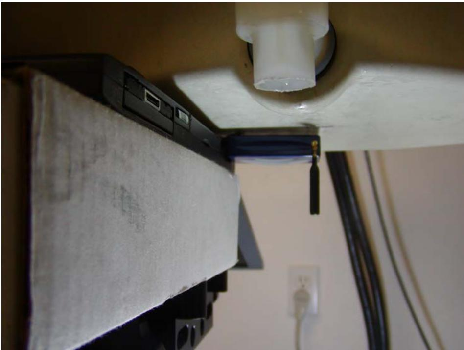
**Toshiba, Bottom Side facing phantom, EUT top side facing phantom, antenna parallel with phantom bottom with headset**
