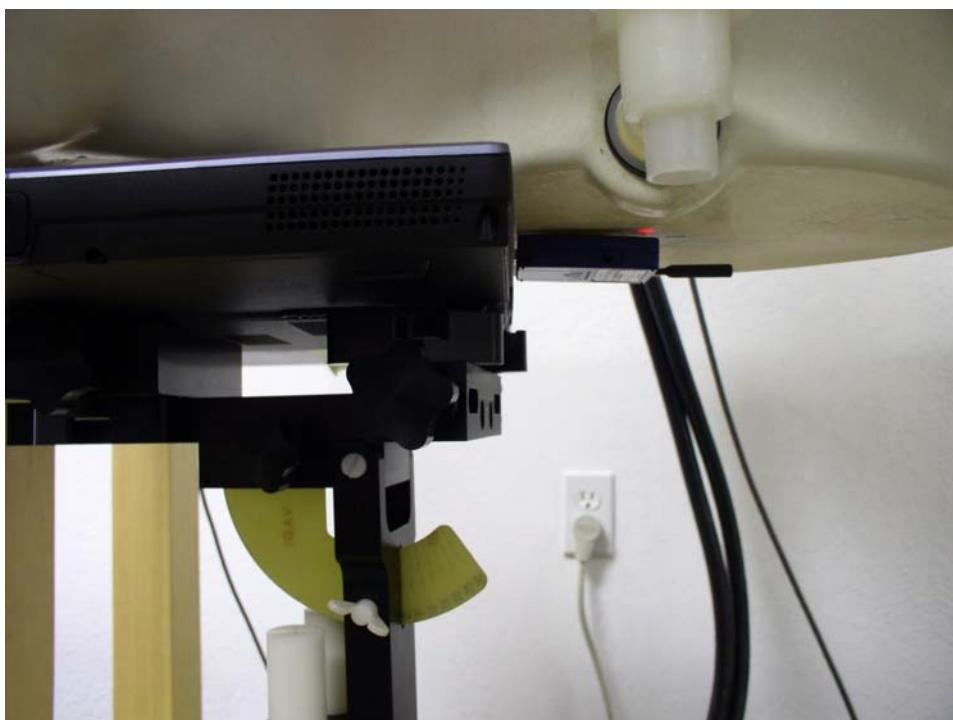
**Compal, Keyboard side facing phantom, EUT top side facing phantom, antenna parallel with phantom bottom (Compal Notebook)**
