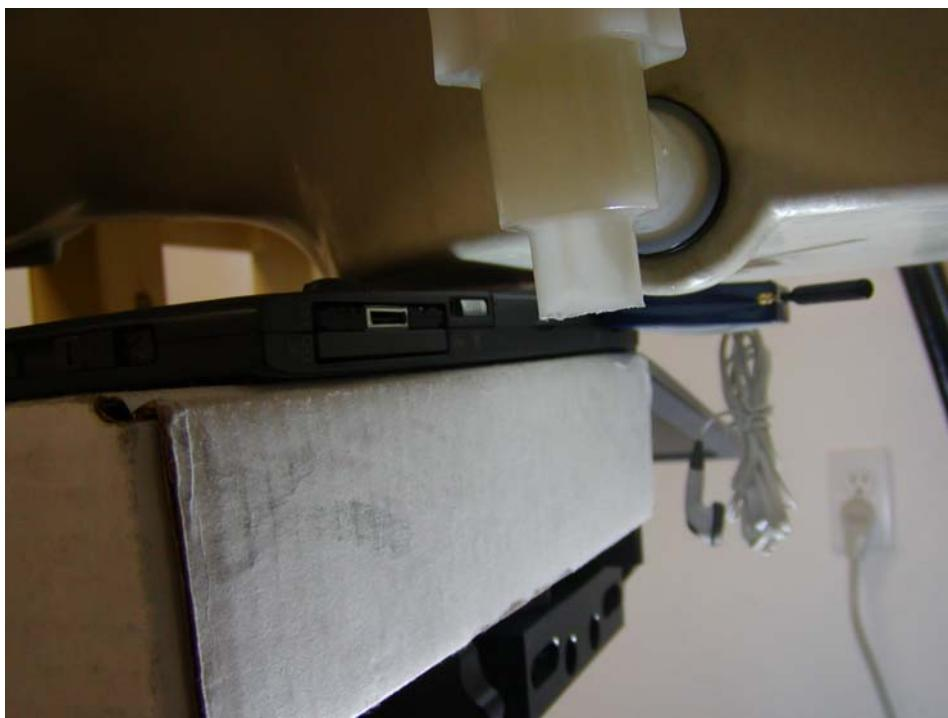
**Toshiba, Bottom Side facing phantom, EUT top side facing phantom, antenna parallel with phantom bottom**
