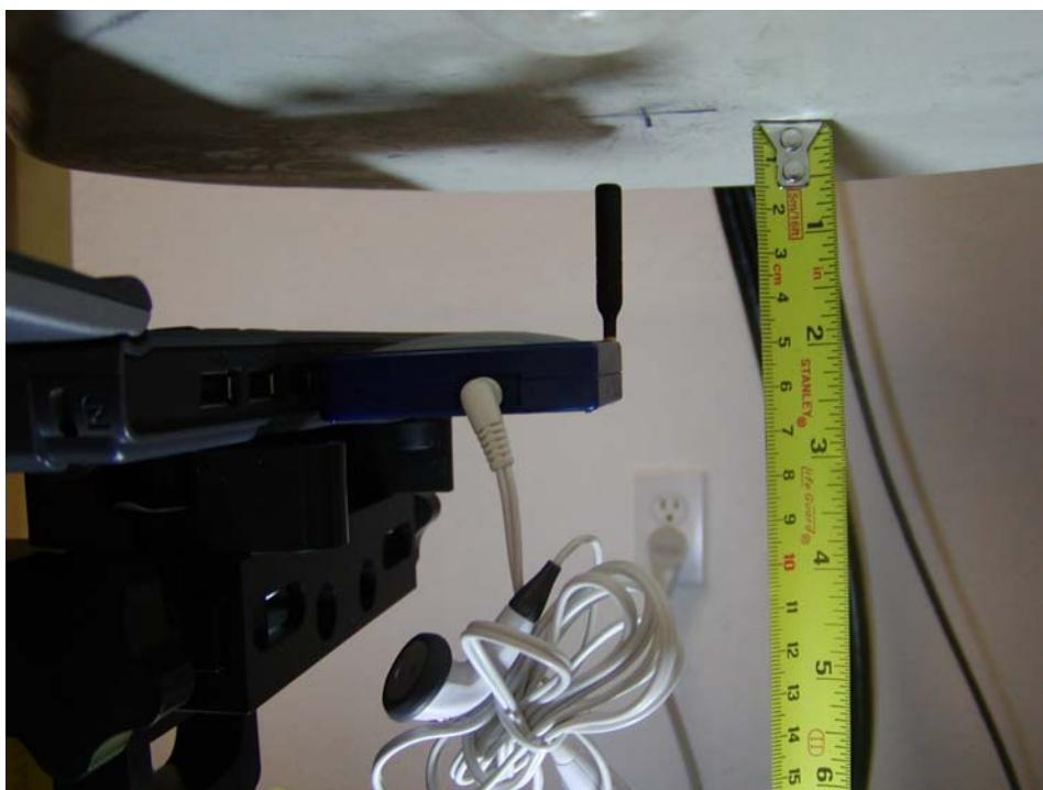
**Acer, Keyboard side facing phantom, EUT Top side facing phantom, antenna pointing into and perpendicular with phantom**
