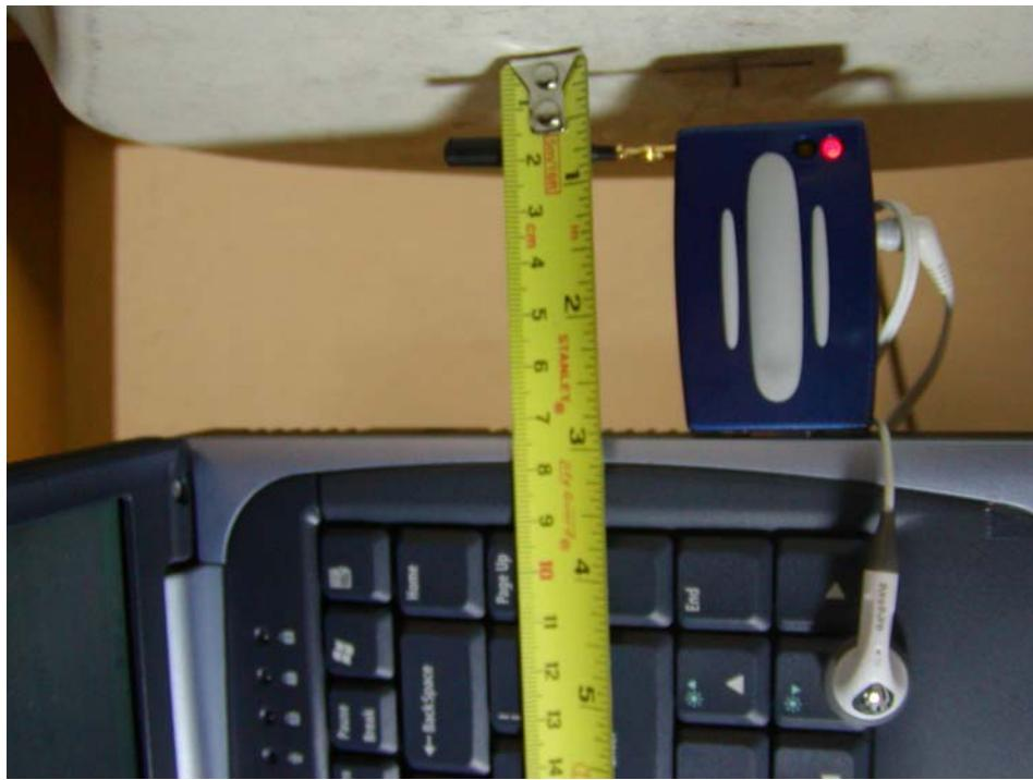
**Compal, left side edge of laptop facing phantom, EUT top side facing phantom, antenna pointing parallel out and perpendicular with phantom bottom**
