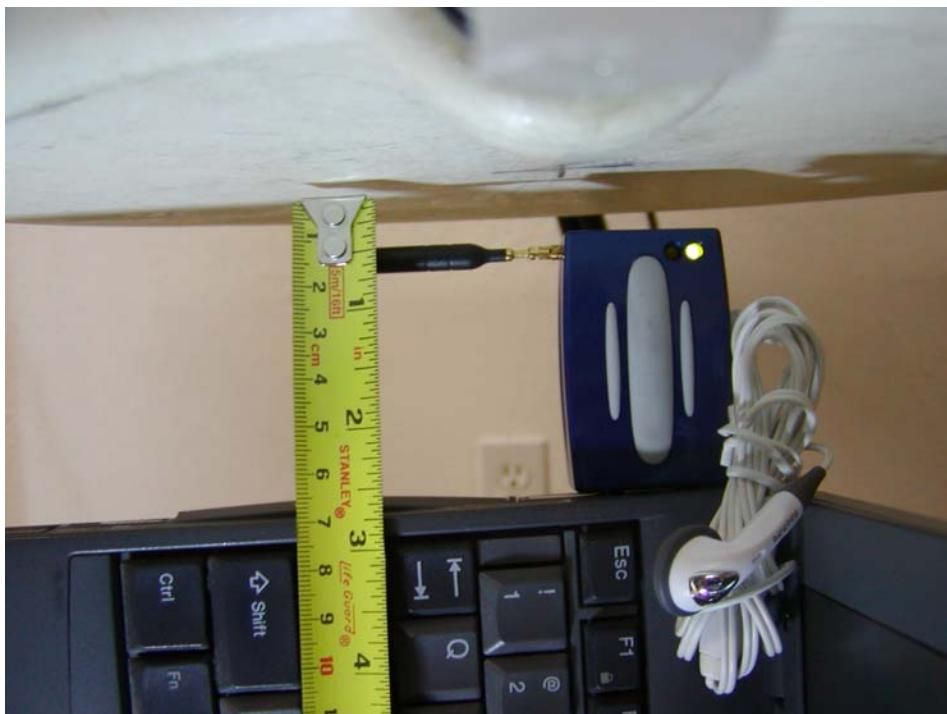
**Toshiba, left side edge of laptop facing phantom, EUT top side facing phantom, antenna pointing parallel out and perpendicular with phantom bottom gaped 1.5cm**
