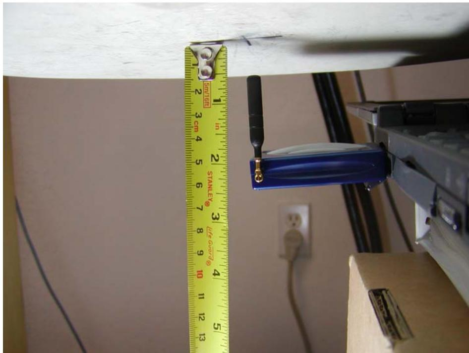
**Toshiba, left side edge of laptop facing phantom, EUT top side facing phantom, antenna pointing parallel out and perpendicular with phantom bottom gaped 1.5cm with headset**
