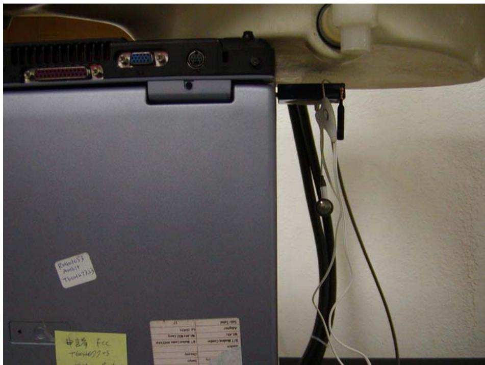
**Compal, Bottom side facing phantom, EUT bottom side facing phantom antenna pointing down and perpendicular with phantom bottom**
