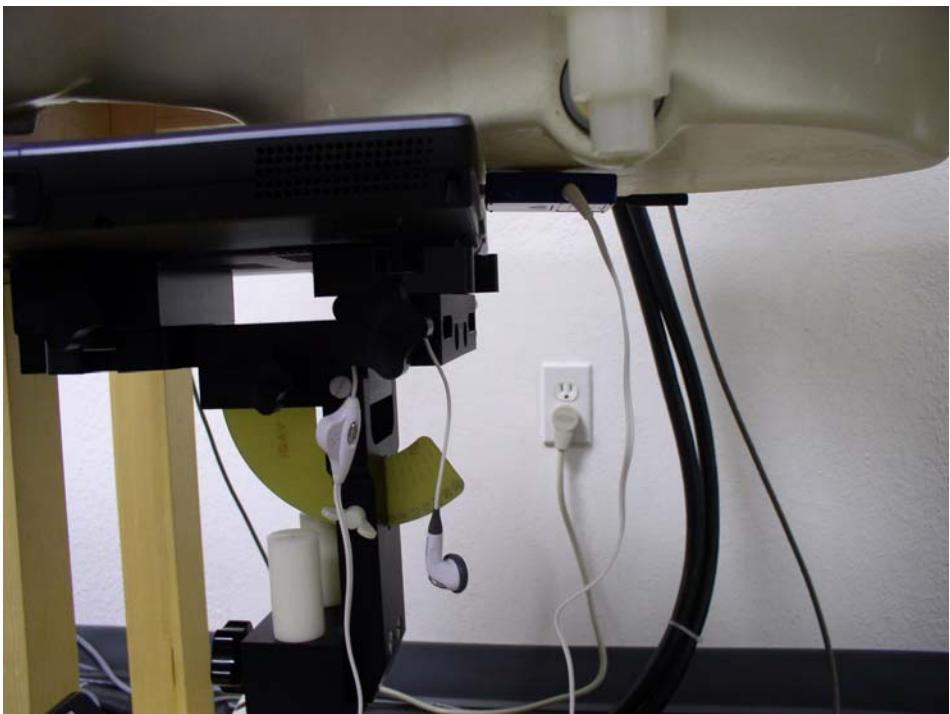
**Compal, Left side edge of laptop facing phantom, EUT topside facing phantom, antenna pointing parallel out and perpendicular with phantom bottom gaped 1.5cm with headset**
