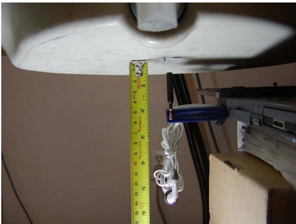
**Toshiba, keyboard side facing phantom, EUT top side facing phantom, antenna pointing into and perpendicular with phantom**
