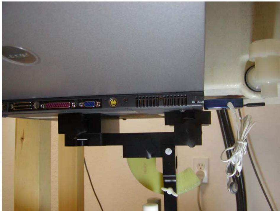
**Acer, Keyboard side facing phantom, EUT Top Side facing phantom, antenna parallel with phantom bottom**
