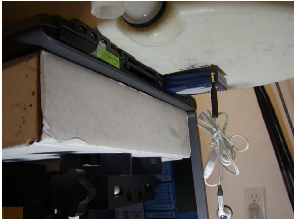
**Acer, Bottom side facing phantom, EUT bottom side facing phantom, antenna pointing down and perpendicular with phantom**
