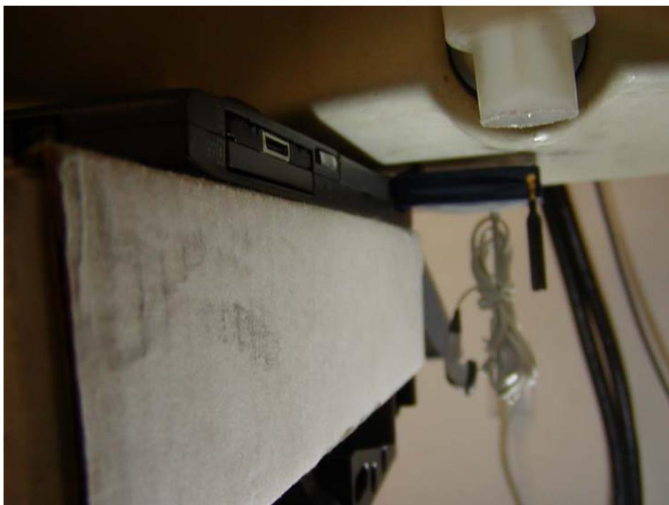
**Toshiba, Bottom side facing phantom, EUT bottom side facing phantom, antenna pointing down and perpendicular with phantom**
