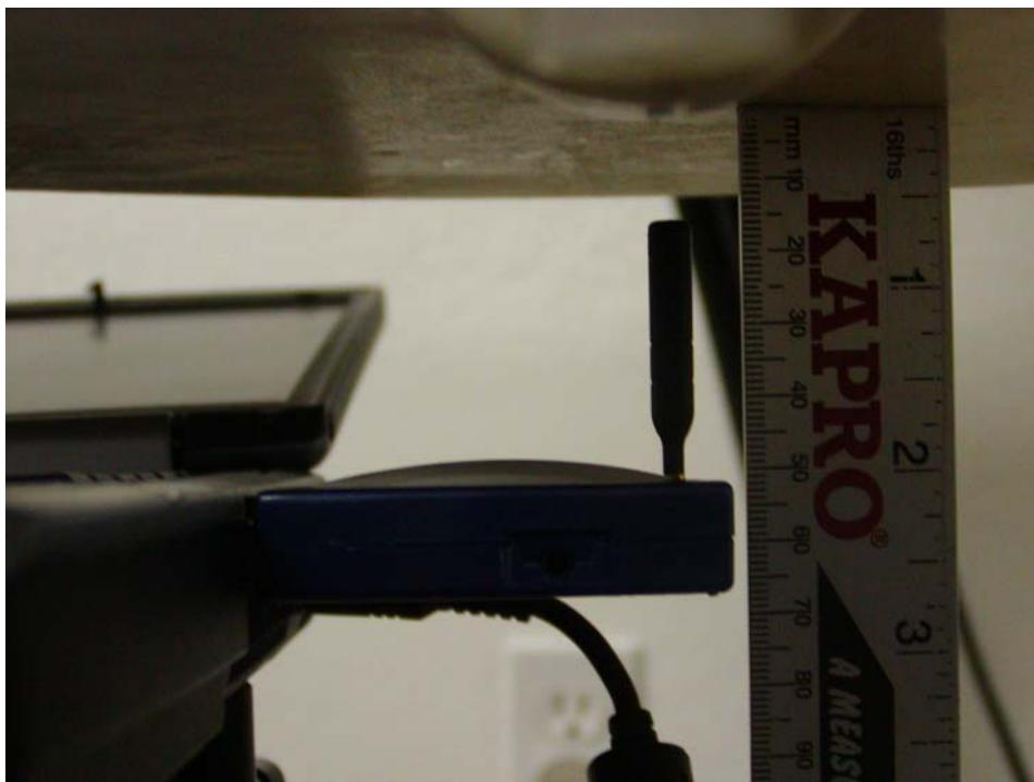
**Compal, Keyboard side facing phantom, EUT top side facing phantom, antenna parallel with phantom bottom with headset**
