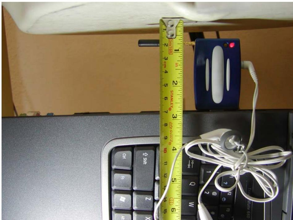
**Acer, Left side edge of laptop facing phantom, EUT top side facing phantom, antenna pointing parallel out and perpendicular with phantom bottom gaped 1.5 cm**
