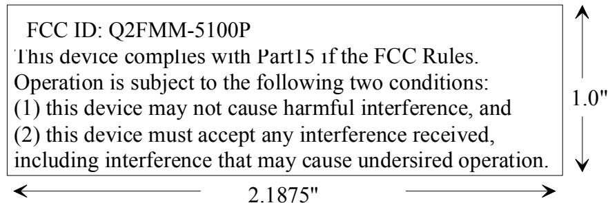
Specifications: Text is black or white in color and is left justified. Labels are silk-screened and shall be “permanently affixed” at a conspicuous location on the EUT.
