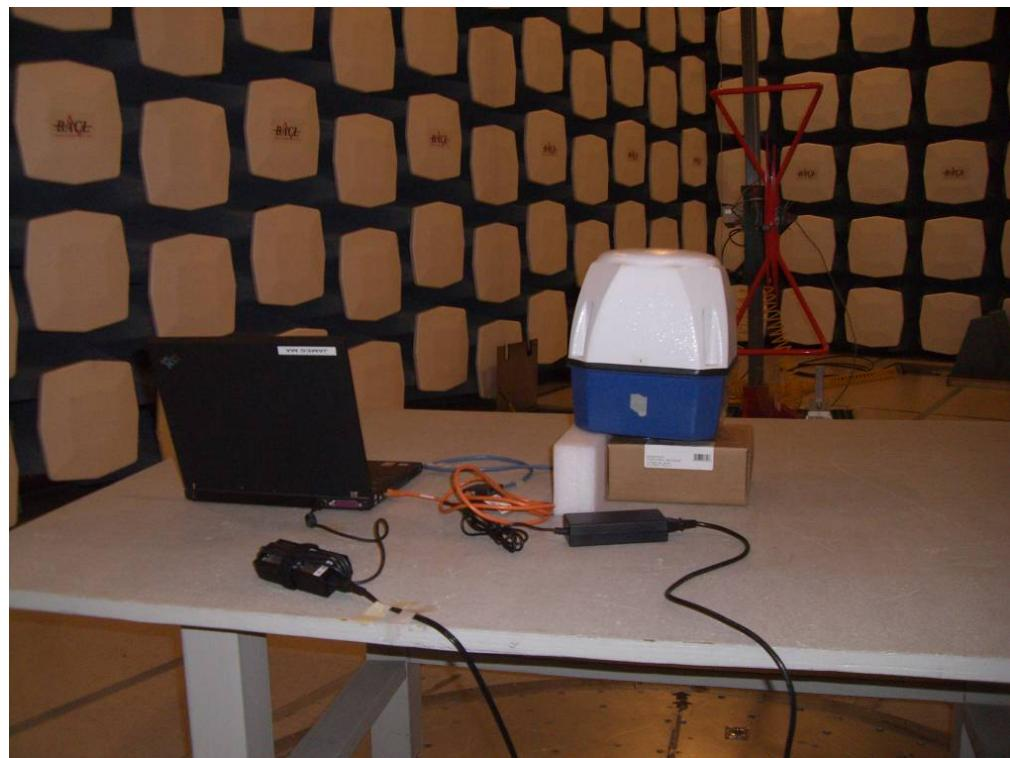
**14.5 Transmitter Radiated Spurious Emissions – Front View**
