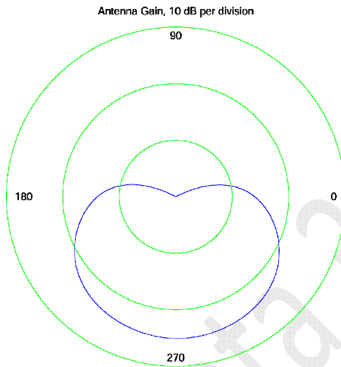
Figure 5 – Sector Antenna Pattern
