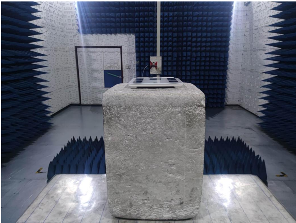
RADIATED EMISSION TEST SETUP ABOVE 1GHz
