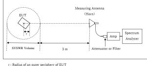
Distance Factor: 20 x log (3.95 m / 3.0 m) = 2.39 dB \* Test Distance: (3 + SVSWR Volume /2) - r = 3.95 m
