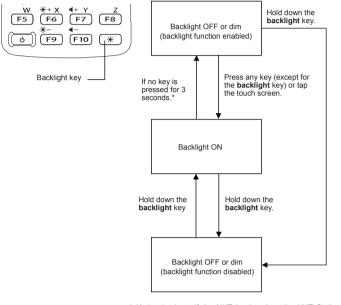
\* Under 1 minute if the HHT is placed on the HHT Station.
