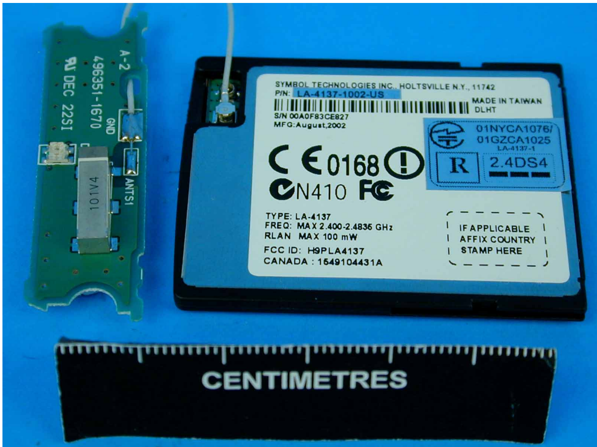
Photograph 2 View of LA-4137 and antenna 496351-1670
