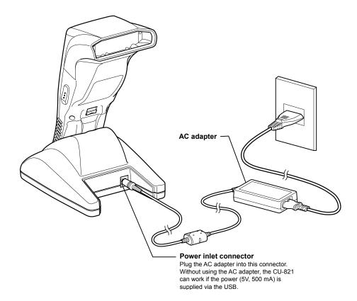
Note: The above diagram is that of the CH-851.
