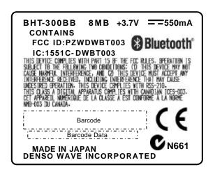
Fig. Label Layout of Scanner Assy
