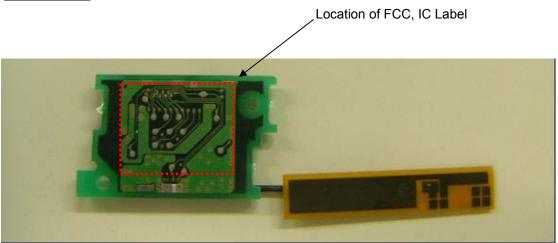
Fig. Photo of Bluetooth Board (Solder side)
