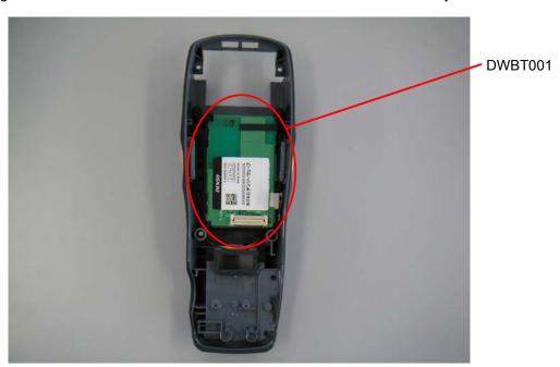
(3) Assembling main circuit board, bar-code scanning module and LCD on lower case of Bar-code Handy Terminal.
