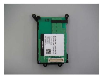
(2) Assembling Bluetooth Board assembled holder in Lower Case of Bar-code Handy Terminal.
