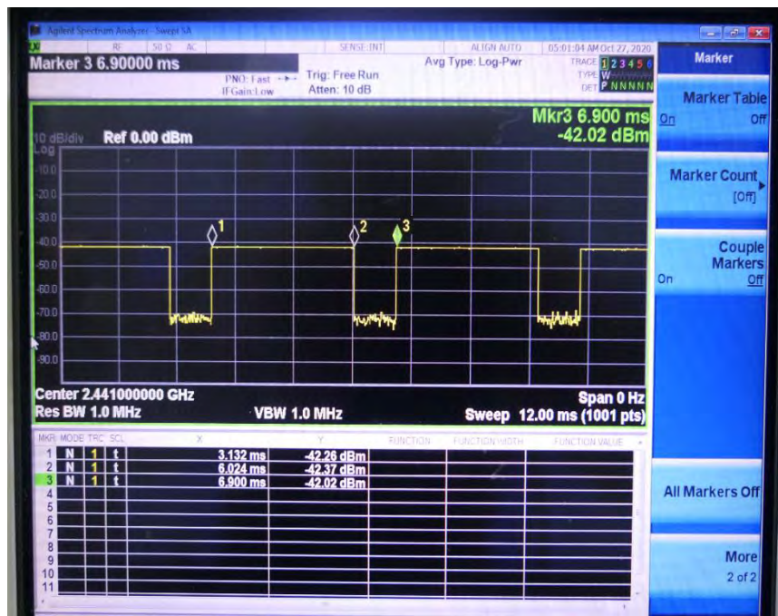
Time-domain plot for Bluetooth transmission signal
