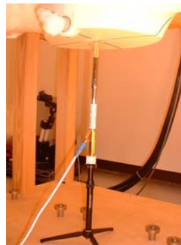
2450MHz System performance check setup
