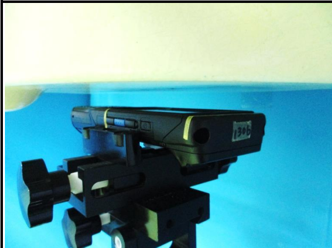
Body worn - Front Face of EUT at 15 mm
