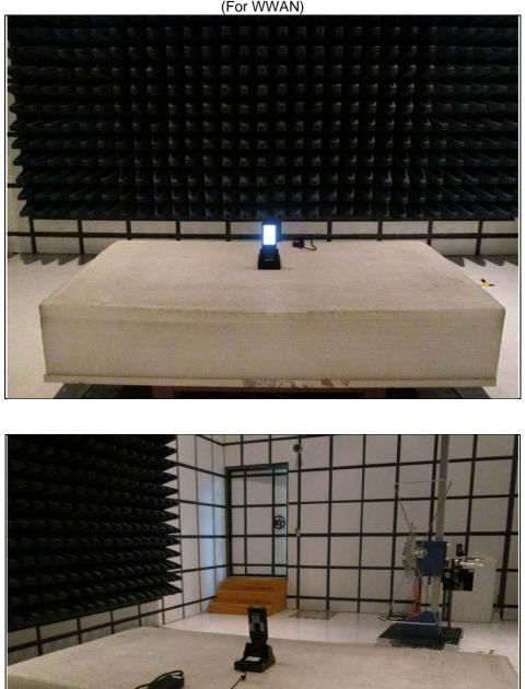
Radiated Emissions (Frequency range below 1GHz) (For WWAN)
