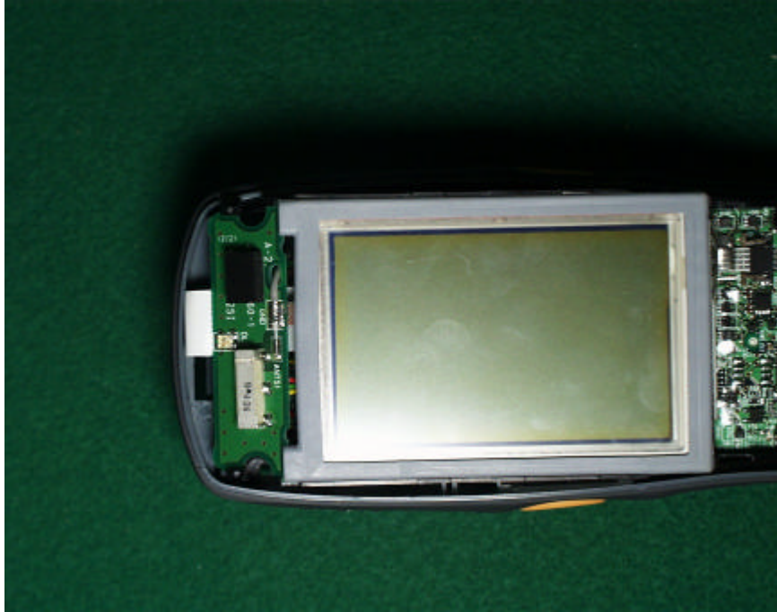
Antenna Circuit Board (Front) and Location
