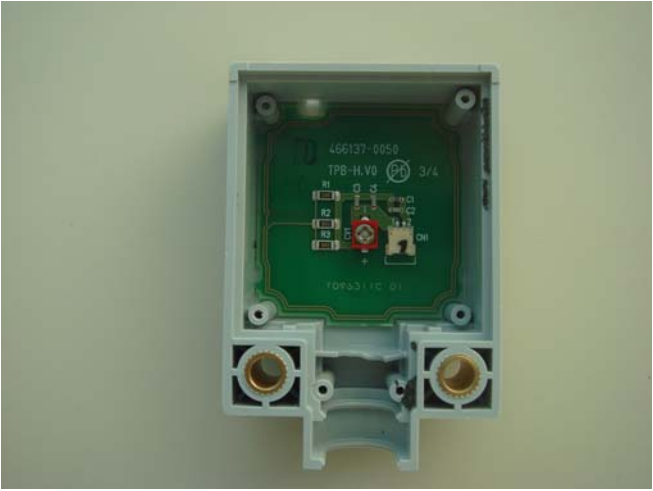
Antenna PCB sub assembly
