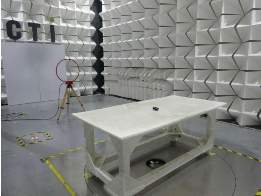
Radiated emission Test Setup-1(9kHz~30MHz)
