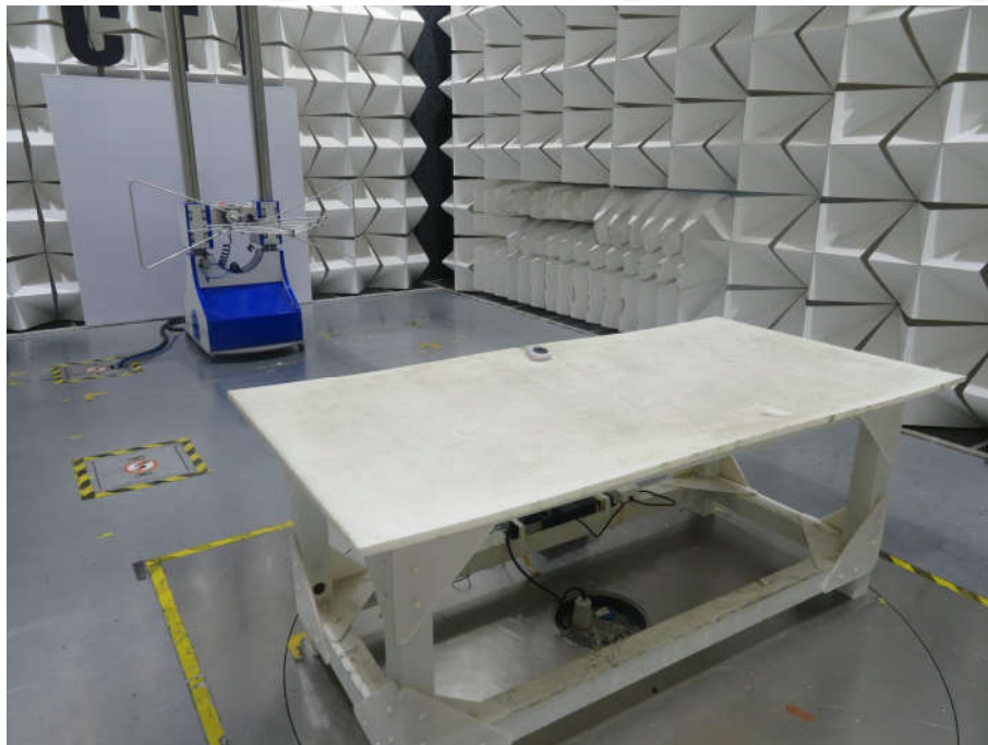
Radiated emission Test Setup-2(30MHz~1GHz)
