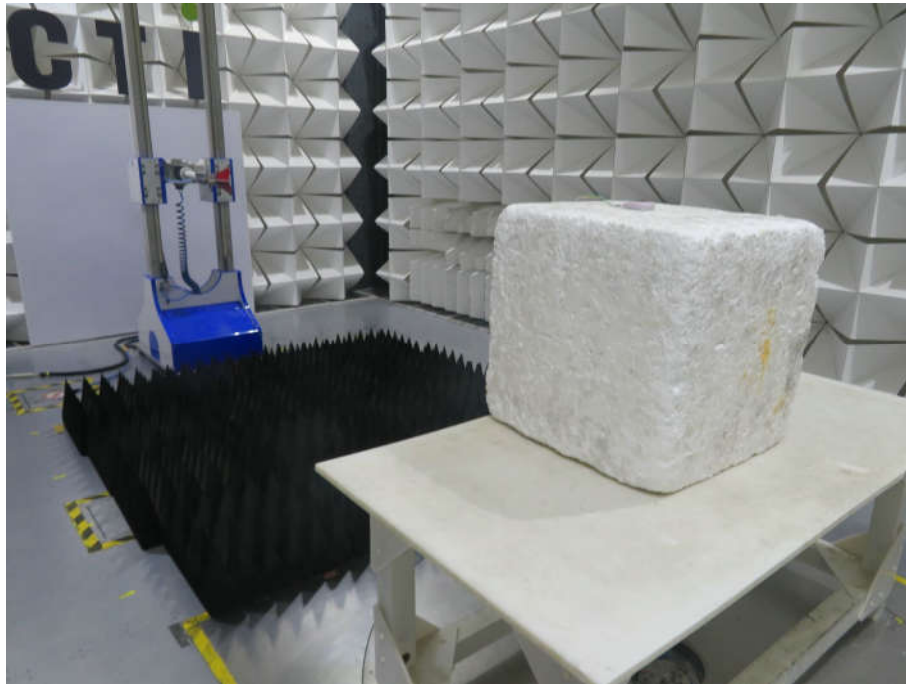
Radiated spurious emission Test Setup-3(Above 1GHz)
