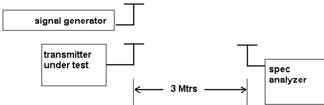
Equipment placed 80 cm above ground on a rotating table platform.
