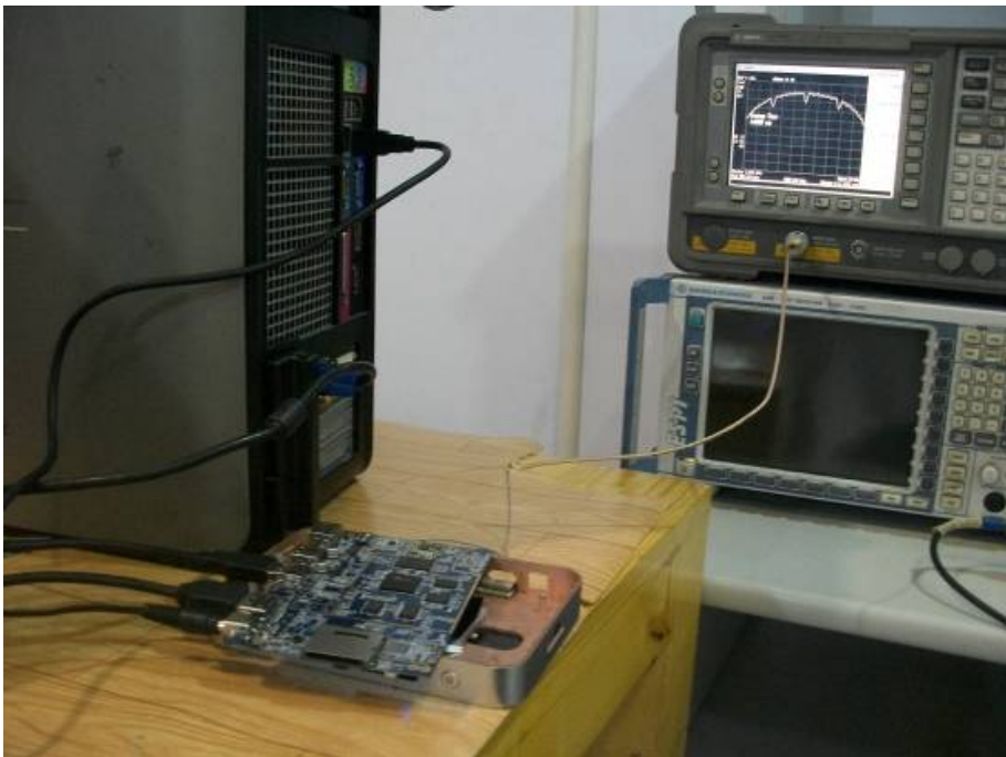
SPURIOUS EMISSION TEST SETUP
