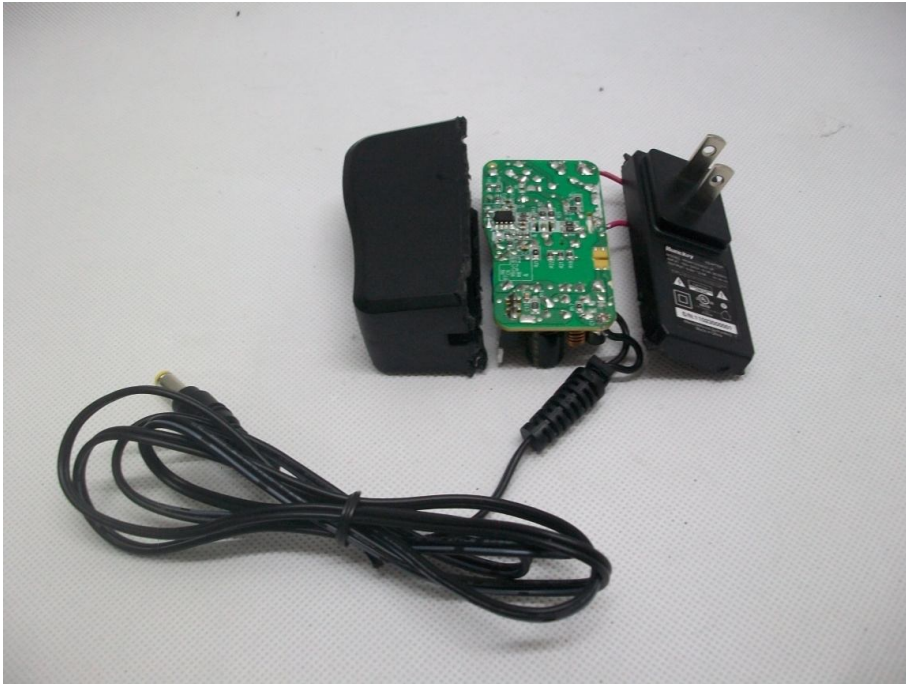
INTERNAL PHOTO OF POWER SUPPLY - 1
